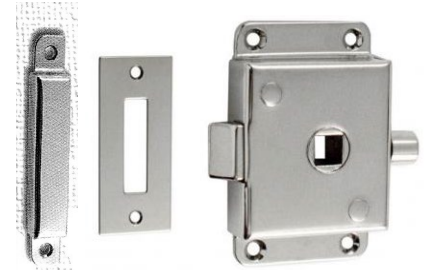
Rim Latch #15.452; Backset 1 1/2" Strike box separate #15.837 Strike plate separate: #15656S For 8 x 8 mm spindle / knobs or levers
